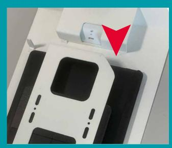
To turn on, locate the power button (indicted by the red arrow) and push for a few seconds.
