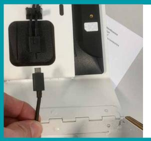
Then feed the power cable through the hole on the rear\* and connect with junction box on lid. You can now clamp the cable internally using clip and connect plug to power supply.
