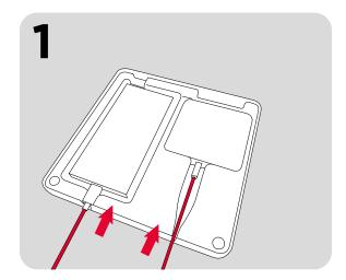
Remove PassBox lid and insert charging cables into phone and SumUp. Cables should sit into channels. Replace lid.
