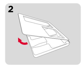
Open the lid by raising the bottom edge to disconnect magnets. Then pull back to un-clip top edge.
