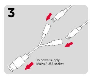
Connect cables to supplied 'Y' extension lead. Lead should then be connected power supply (not included).
