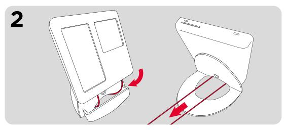
Seat PassBox on the base unit allowing cables to pass through top or the holes (depending on base model) and through rear opening. The PassBox can now be located on the base using rear holes & base unit mounting screws.
